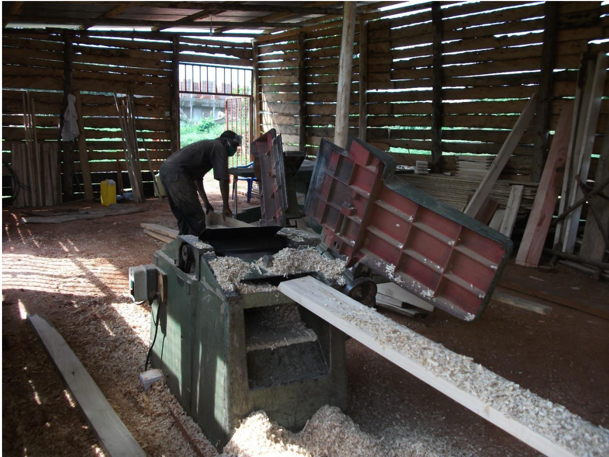
Work in progress, timbers being feed to the machine for thicknesses
